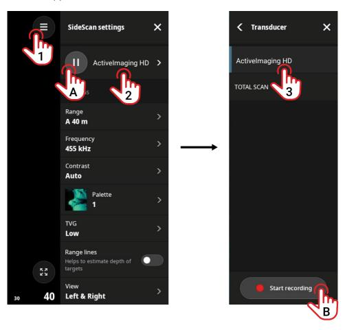
Select the pause button (A) to pause the transducer from transmitting. The system does not collect data when the transducer is paused.
