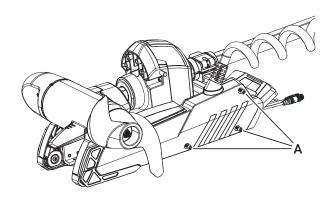
Remove the side plates, taking care not to damage the locating tabs as they leave their slots (**B**).
