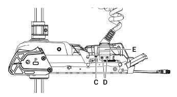
7 Lift the UI cover upward to separate it from the mount.
