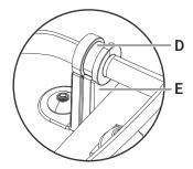
**4** Lower the mount UI cover into position. Guide its front face to fit over the cable retainer and grommet.
