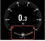
→ Note: V12 engines have an integrated gearbox, hence the engine speed and prop rotation speed are not the same. The gauge displays the engine speed. In Cruise control mode, the target RPM is the propeller RPM. The engine gauge displays engine RPM, so the two RPM values can differ when cruise is active. This is normal.
