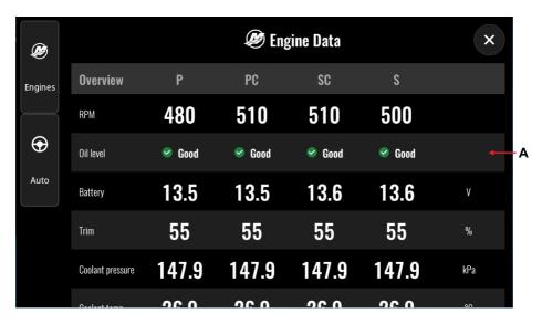
Some engines can carry out an oil level check on request. This is referred to as an active oil level check. If your Mercury engine supports the feature, select the **Check** (**B**) button to initiate it.
