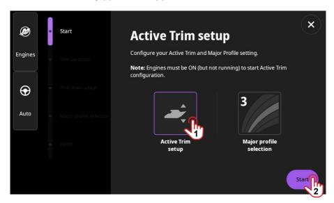
Follow the on-screen prompts. The trim position shown on screen changes as the engine trim changes. At the end of the range of motion, continue to hold the engine trim button for 5 seconds, to set.
