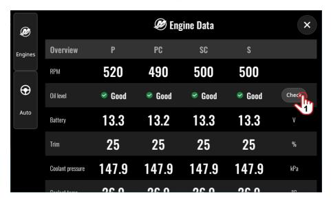
During a check the engines will move to a level position, and may throttle up to reach the correct temperature and pressure for the check.
