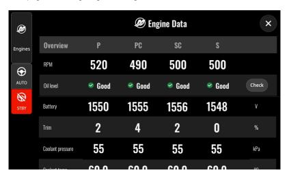
→ Note: The data includes engine-specific details such as trim and steering, among other features. Each row displays data only if the engine(s) can provide it.
