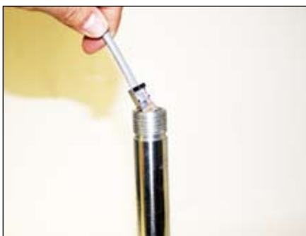
Insert RJ45 Interconnect Cable into mast/pole mount.
