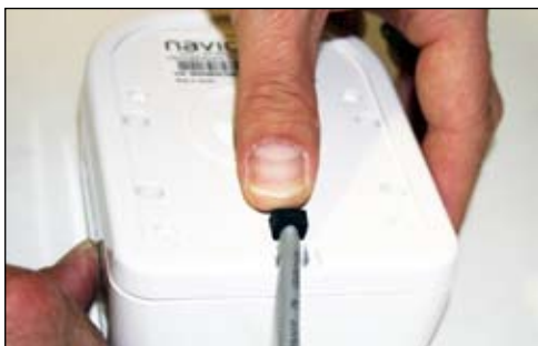
Insert rubber boot into boot inset.
