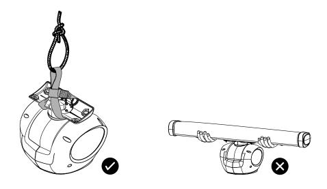
Marning: Do not lift the pedestal with the antenna attached.
