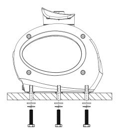
If you're installing the pedestal onto a steel surface, also use the supplied plastic isolating washers.
