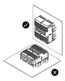
The RI-50 must be located where it can easily connect to the vessel's ground connection, the pedestal interconnection cable and the power cable.
