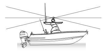
If you install your HALO radar on a power boat with a steep planing angle, it is recommended you tilt the radar angle down at the front.
