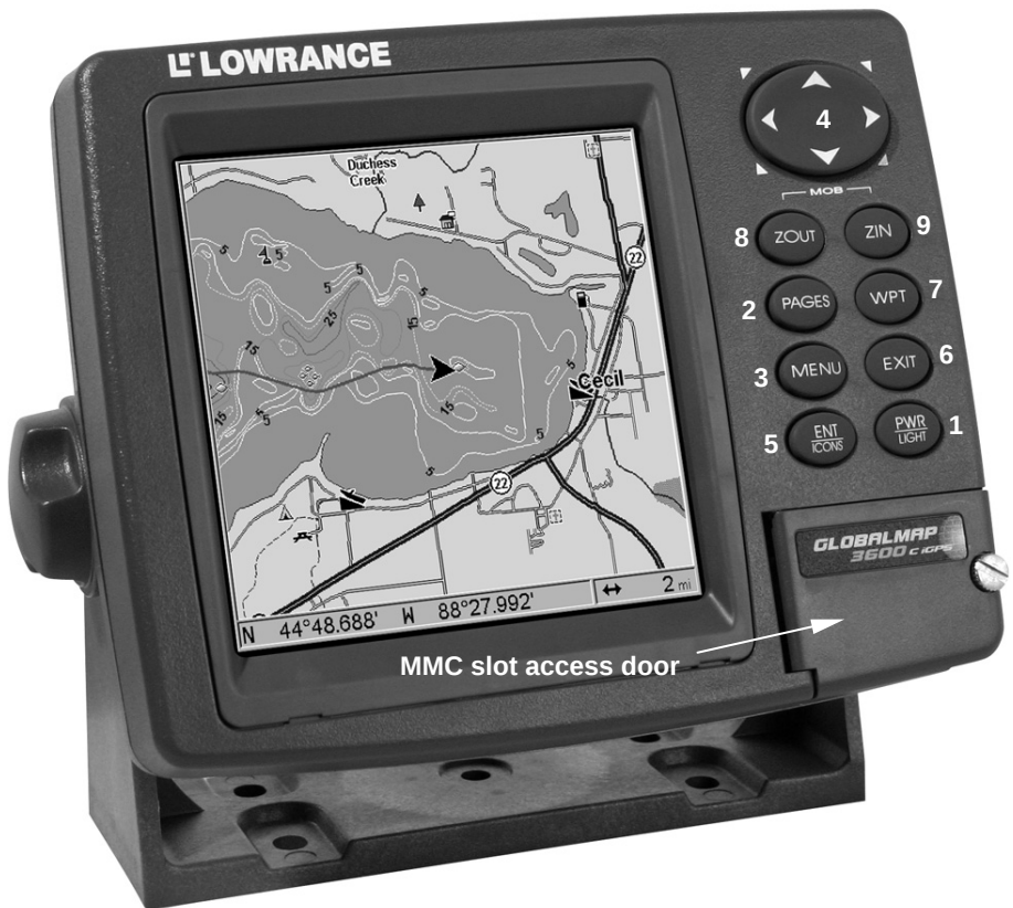
GlobalMap 3600C GPS unit, front view, showing Map Page, keyboard and access door for the MMC slot.
