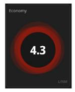
Red – Poor economy Vessel is running inefficiently compared to target. Vary throttle and check target efficiency.
