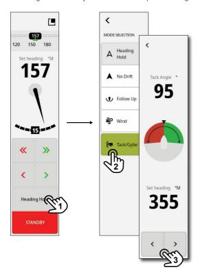
→ Note: The tack angle and rate of turn during the tack/gybe are set in the autopilot sailing settings.
