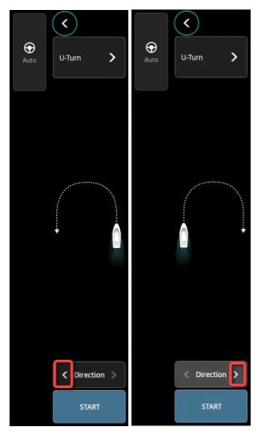
→ Note: You can adjust the turn rate under Autopilot settings > Tune Autopilot > Rate Limit.
