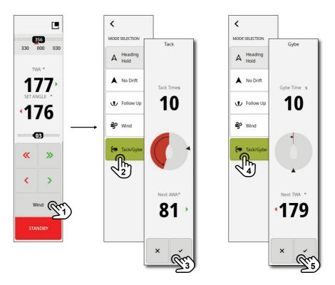
→ Note: The autopilot will temporarily add a 5° bear-away on the new tack to allow the boat to pick up speed. After a short period the wind angle will return to the set angle.
