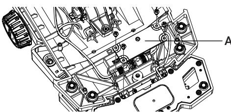
→ **Note:** The lower key module is now unsupported and attached only by a single connector.
