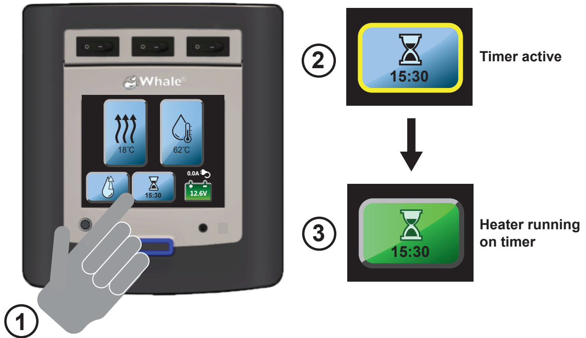
Figure 7. Whale® iVan Control Panel - Activating Water Heater Timers
