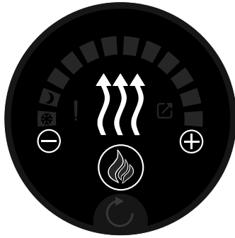
Figure 1. Whale Heat Control Panel
