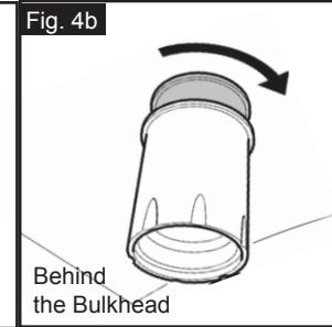
**STEP 3** Place the housing through the hole. Secure by hand tightening the lock nut onto the housing behind the bulkhead. (See Fig. 4a and 4b)
