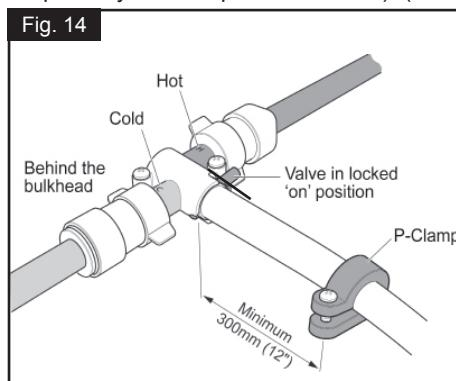
**STEP 2** Screw p clamp to bulkhead ensuring it is located at least 300 mm (12") from the valve housing (See Fig. 14).
