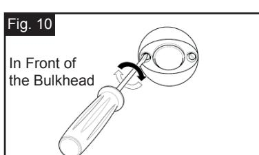
**STEP 5.** Place the housing through the hole (Fig. 9). Install by tightening the 2 screws in the front face until the flange is securely mounted to the bulkhead (See Fig. 10) i.e. touching at all points around the circumference. Ensure that the screw holes are on a horizontal plane.
