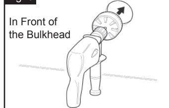
**STEP 3.** To enable ease of fitting of the holder and support rings, the two screws should be loosened until almost disengaged from the threaded part.
